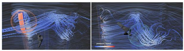
Figure 1: *3De lens* inspecting wind turbine aerodynamics. (*left*) The lens depicts strong-pressure gradient on the leftmost wind turbine blade; it also selects the air flowing around this blade and advancing to the rightmost one. (*right*) By setting its orientation, the lens selects a disorderly bundle of flow lines passing through the central blade.
